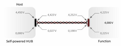
Bus topology under the maximum acceptable voltage drop
