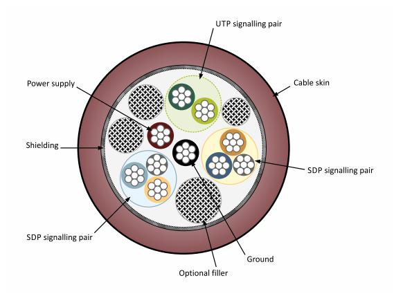
Cross section of cable in USB 3.0 specification
