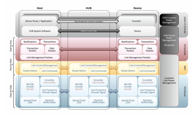
Communication layers of SuperSpeed bus
