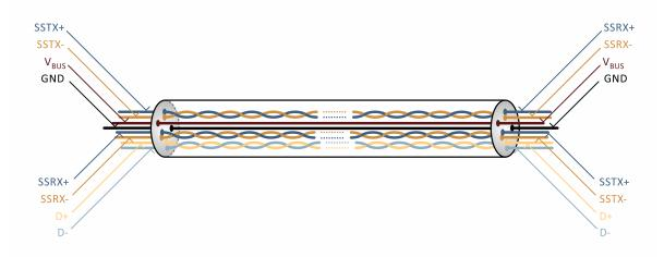
Diagram of cable in USB 3.0 specification
