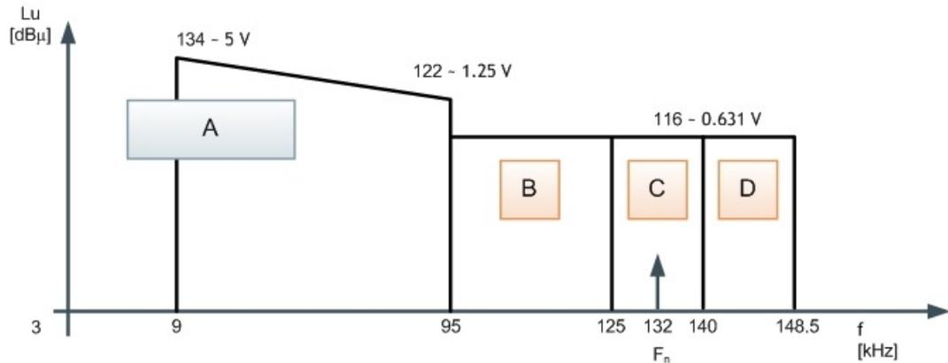
Frequency bands and limit values of the output voltage.
