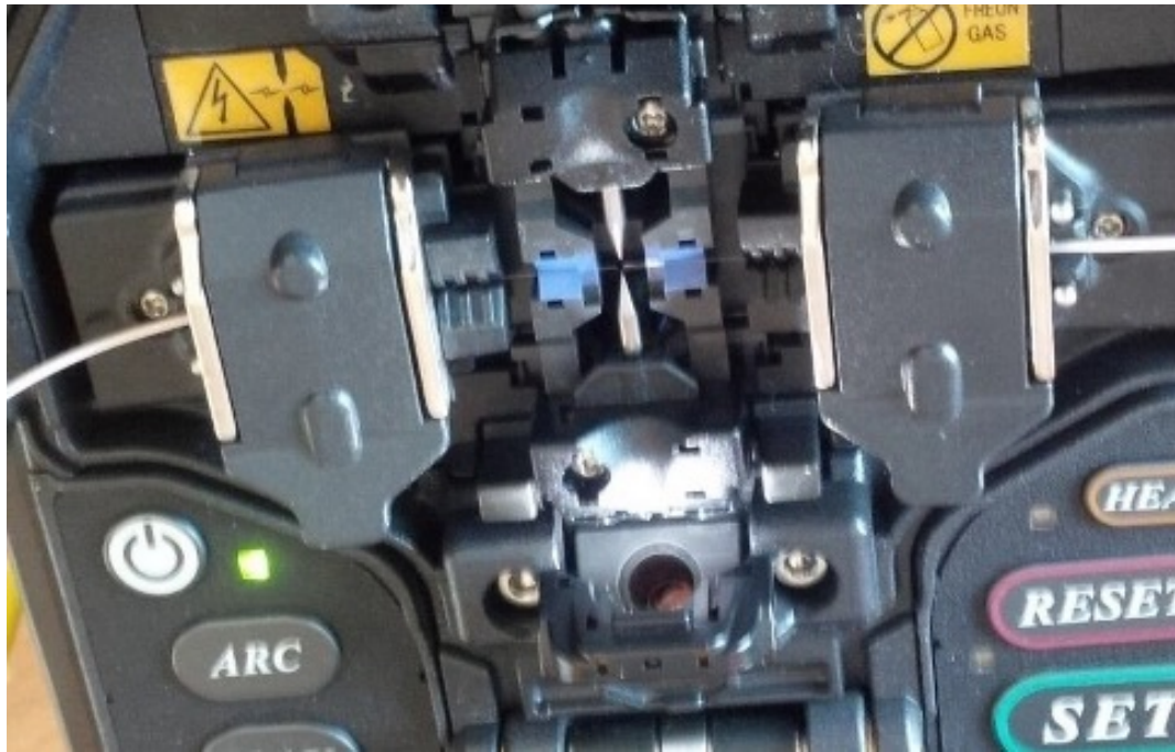
Splicer with fibres positioned close to the electrodes in the centre, held in place by spring-loaded clamps.
